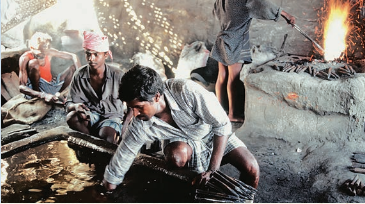
3 Blacksmiths at the worksite manually sharpen steel chisels by the hundreds every day for the stone carvers
